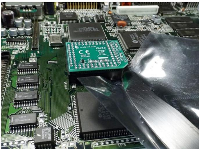
KA21 may be dismounted with some thin, stiff, but not sharp tool, like butter knife or small flat screwdriver. Put some paper (or ESD bag, like on the photo) under the tool, to avoid mainboard scratching. Then insert the tool edge into the gap between KA21 socket and the mainboard. Pry up the socket on a corner. Then carefully remove KA21 by hand, pulling it up. Do not use excessive force, pry up the opposite corner if needed.
