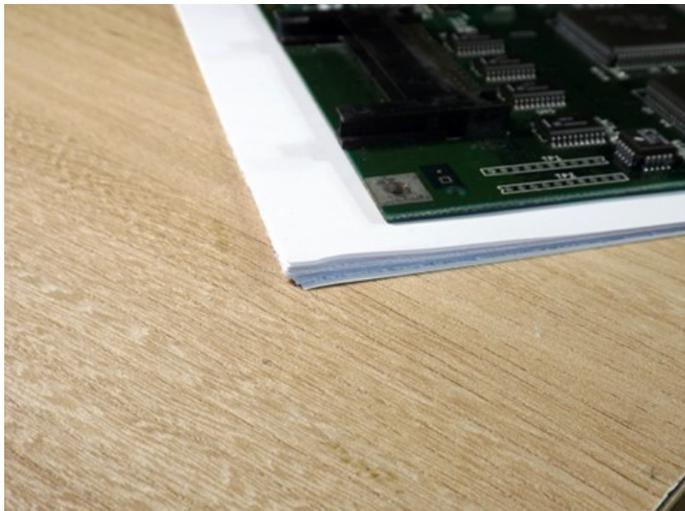
**Step 3:** Put the mainboard on ESD mat (the best), stack of paper, a newspaper or cardboard, to give even support under the Gayle chip. Do not use plastic materials like foam or bubble wrap, as they easily generate electrostatic charge.
